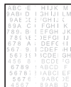
Print is faded or vertically aligned white streaks are apparent (see page 150)
